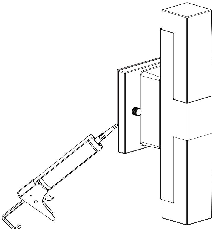
**NOTE:** We recommend keeping the bottom unsealed. To maintain a drainage area in case of water infiltration.
